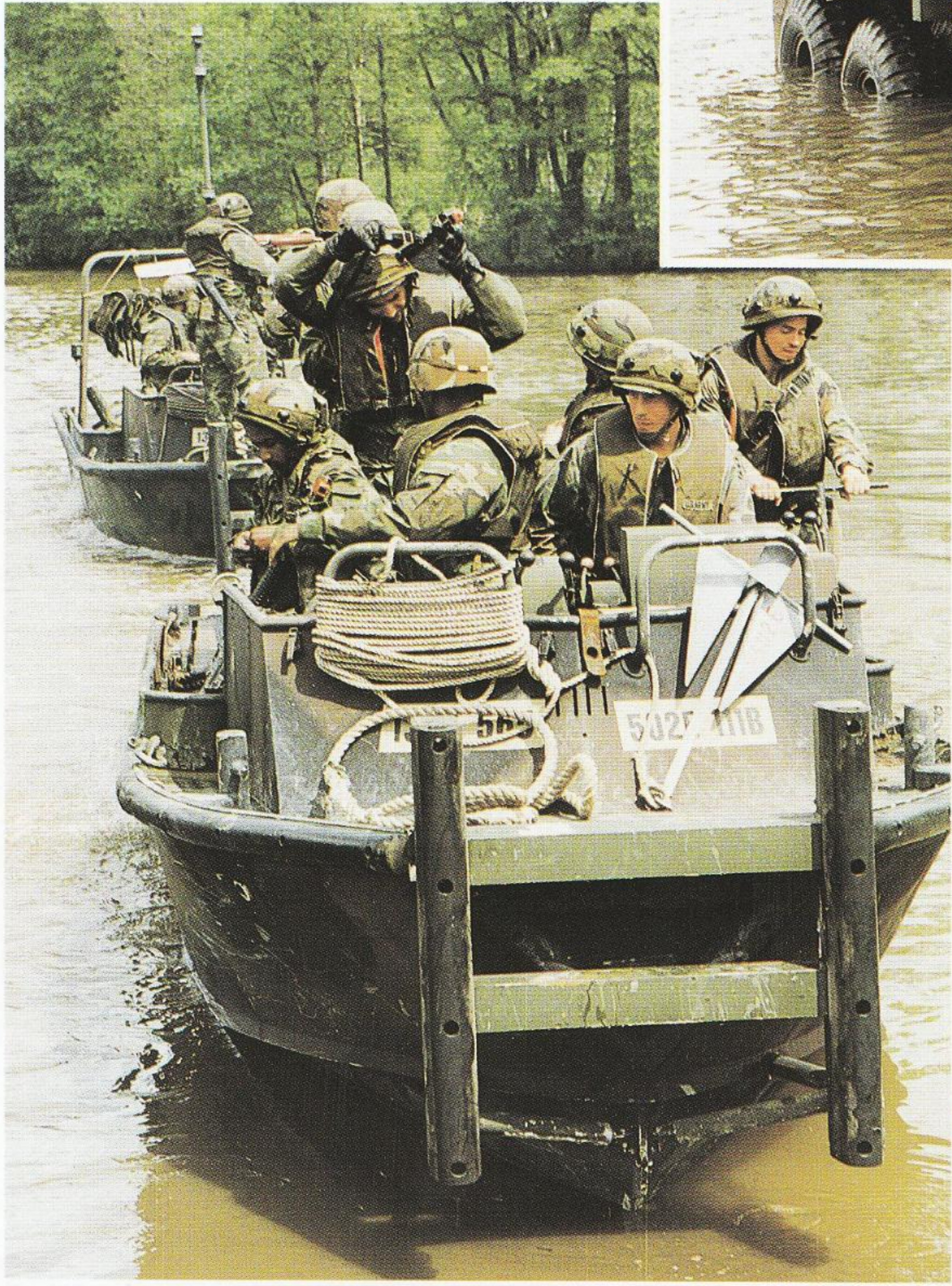
Assault bridge boats from 502nd. Engineer Co. drive into position and wait for the ramps and interior bays. The boats hold the floating bridge in place. The safety boat is used for security and first aid purposes.
