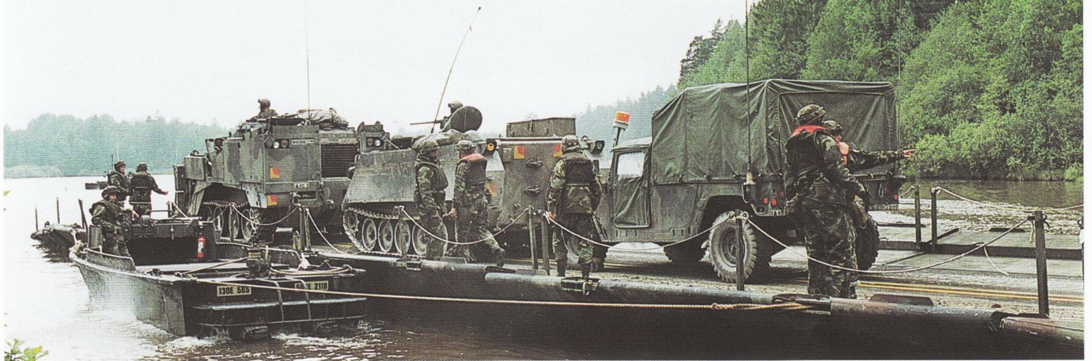
RIBBON-BRIDGE in use as a ferry raft with engineer vehicles as M9ACE, M113 A3 and Humvee of the 40. Combat engineer Battalion. The RIBBON-BRIDGE system was first fielded by the US ARMY in West-Germany and South Korea in 1976. The equipment of the 502. Engineer Co. consists of 30 interior bays and 12 ramps, sufficient for 212 meters of fixed bridge or six 70 ton rafts.
