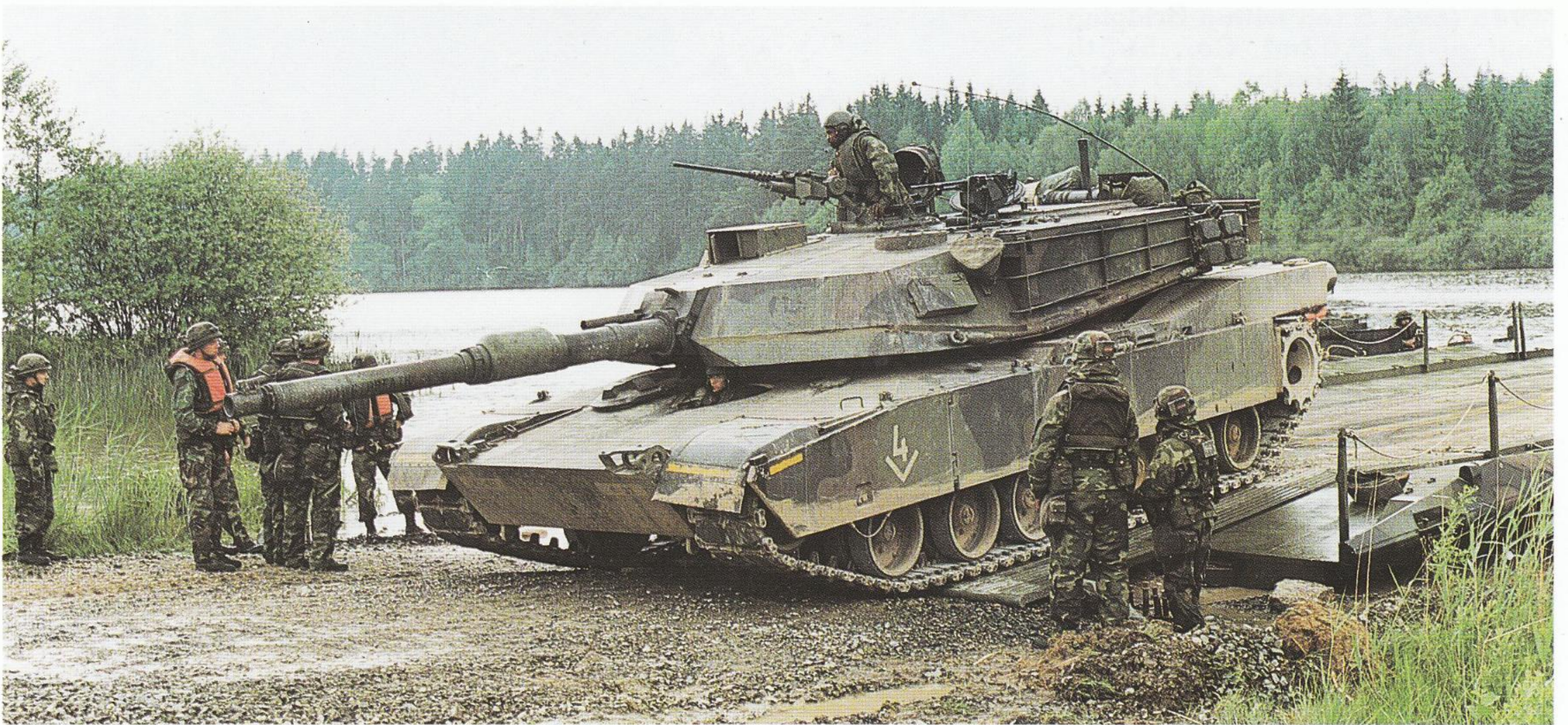
M1A1 HA Abrams from 2 Bn., 68th Armor Rgt. leave a RIBBON-BRIDGE tank ferry. The Bridge can support 70 ton loads and 80 tons when conditions are ideal.
