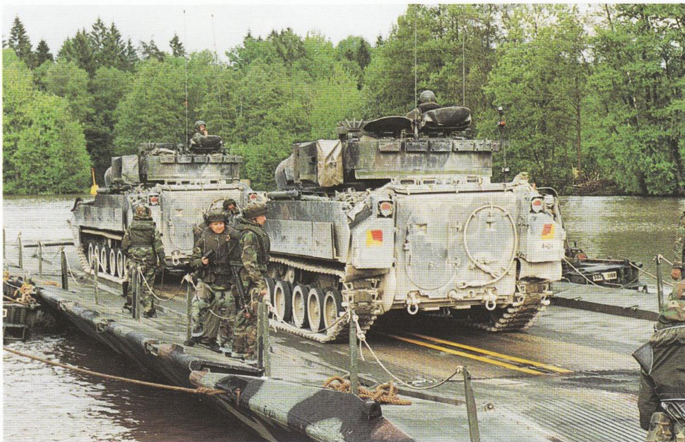
M1A1 HA Abrams from 2 Bn., 68th Armor Rgt. leave a RIBBON-BRIDGE tank ferry. The Bridge can support 70 ton loads and 80 tons when conditions are ideal.
