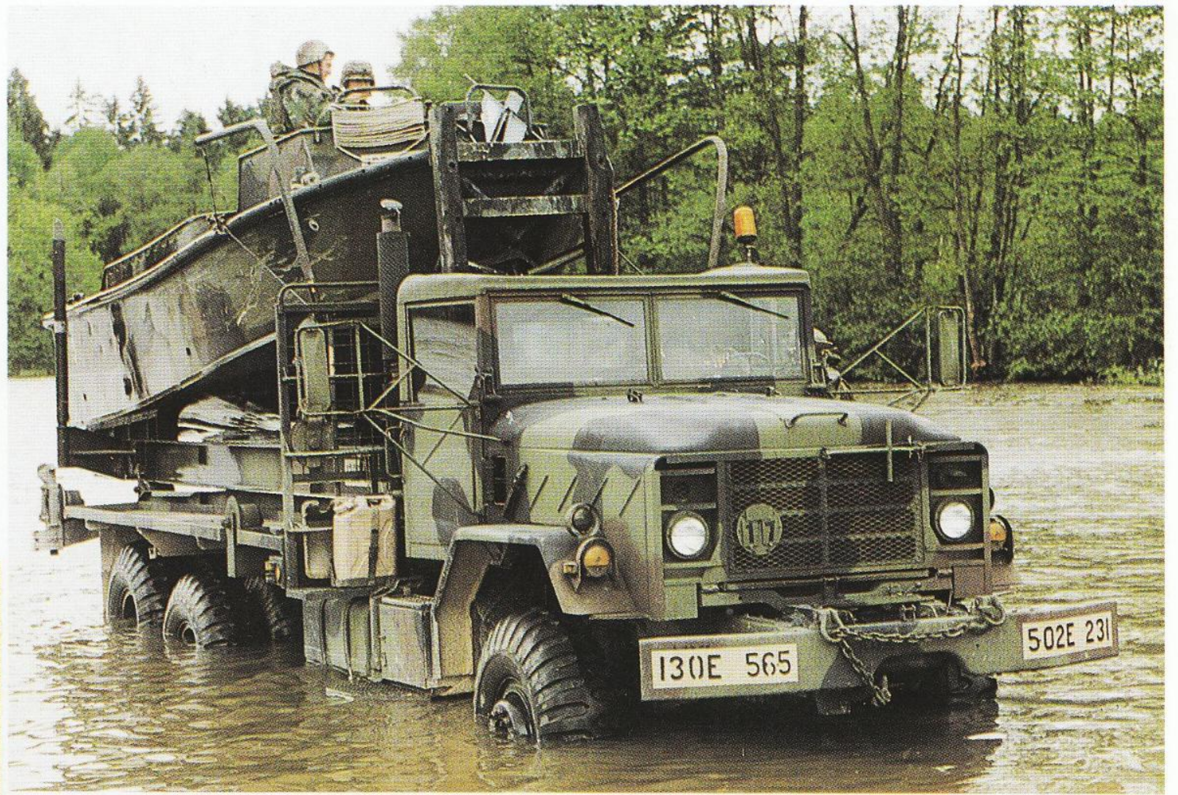
M945 (6x6) 5 ton with a Bridging Boat of the 502nd. Co., 565th Engineer Bn., during "RAFTING OPERATION" at Grafenwöhr swim site.
